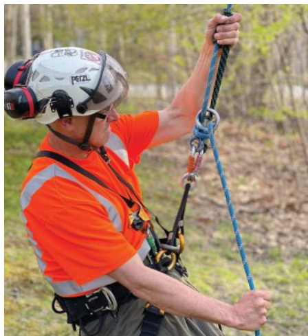
Photo 3: Figure-8 descender with Prusik loop backup.
