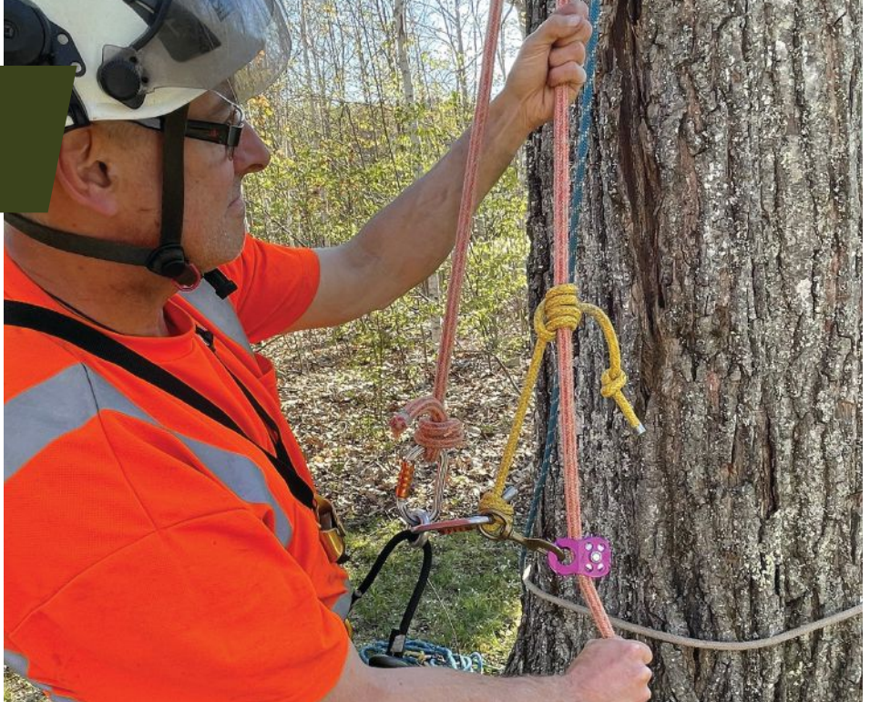
Photo 1: The author employs a split-tail climbing system. Unless otherwise noted, photos by Rebecca Gard, courtesy of the author. In the photos with this article, the author is shown inspecting his climbing system prior to ascent, and for that reason has not yet lowered his Z87-approved visor.
