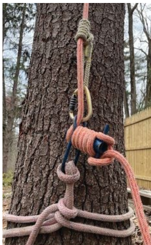
Photo 5: Mini Port-A-Wrap with a Prusik backup.
