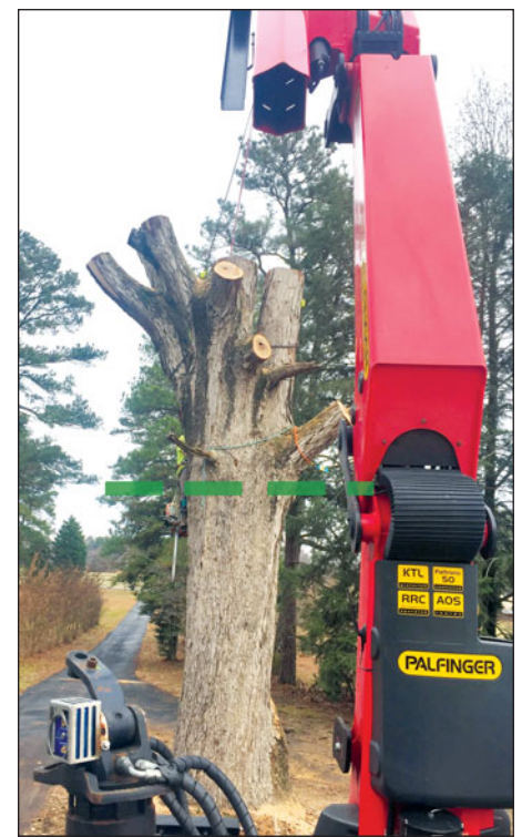
Photos 4 & 5: From my vantage point on the ground, the location of the cut appeared to be low enough into trunk wood to prevent any separation of the leads coming together on the base of the cut.
